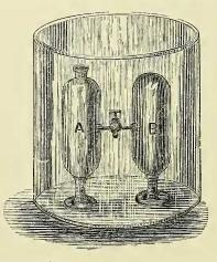
When the experiment is finished it will be found that there is no change in the temperature of the water. The prevalent idea is that when air expands it becomes colder, and that when condensed it becomes hotter; but Joule, by this experiment, has shown that no appreciable change of temperature occurs when air is allowed to expand in such a manner as not to develop mechanical power."
